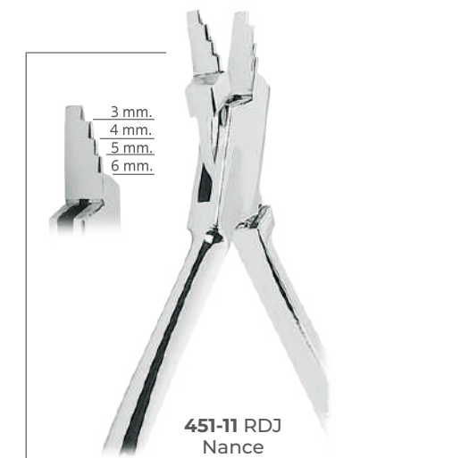
Nance Loops Closing Pliers Nance Style. With 4 Steps Tip For Forming Various Size Loops In Rectangular And Round Wires, Up To 0.7 mm (.028")
